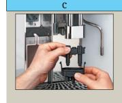
\* Rinse combi spout and milk hose very thoroughly with clear water so that no cleaning fluid remains
